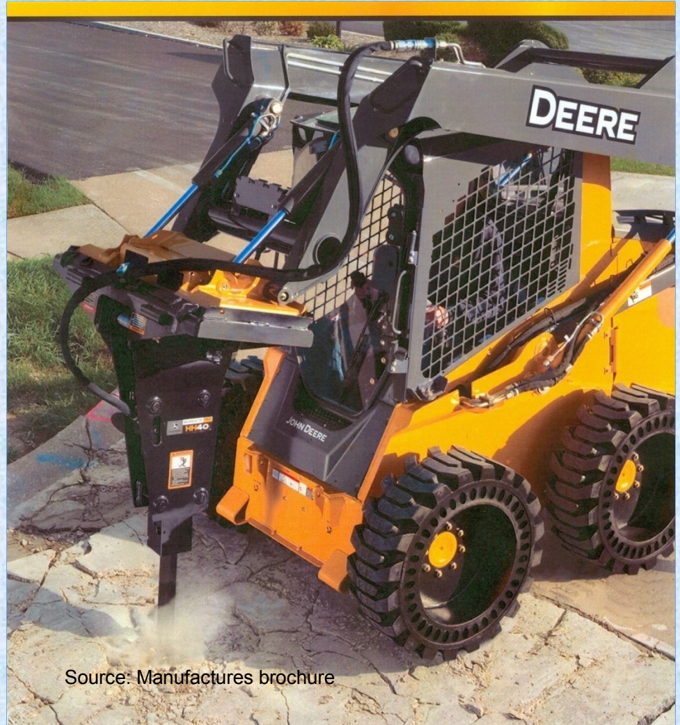
Hydraulic hammer with chisel mounted on a skid tractor
